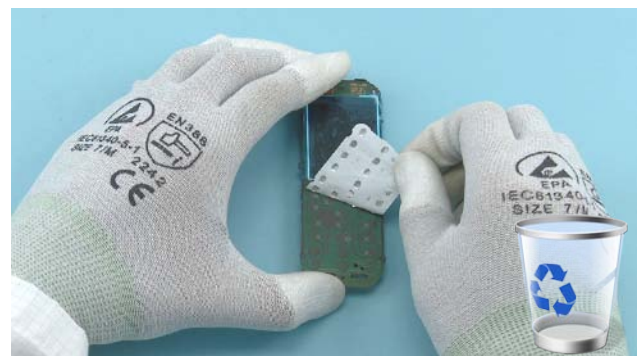
18) Peel off and remove the DOMESHEET. Do not use it again. Discard it.
