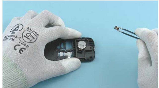
20) Remove the DC JACK with the tweezers.
