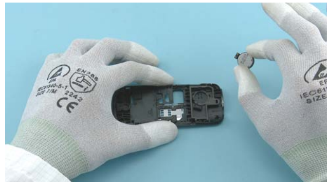
22) Remove the EARPIECE/SPEAKER/VIBRA.
