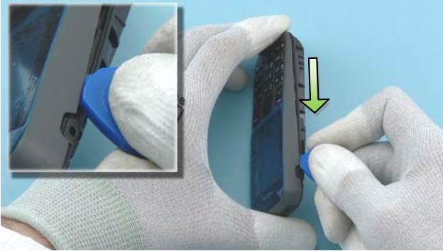
7) Open the left side of the A-COVER by sliding the SRT-6 to direction shown.
