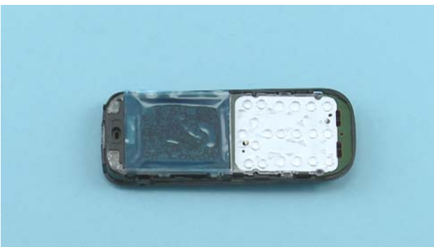
11) Protect the DISPLAY with protective film.
