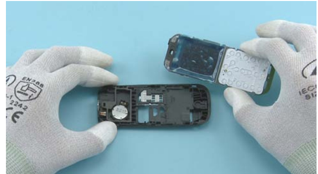
14) Remove the ENGINE BOARD.
